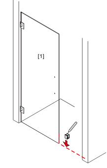
5. Draw a line along the center of the Door Panel[1] side, extending to the floor. Position the Bottom Clip[14] and make a mark on the floor through the hole of the Bottom Clip[14] for drilling. Drill holes with a φ0.24" drill bit, insert Wall Plug[16] and secure the Bottom Clip[14] to the floor with Flat Head Screw ST4x25[15].
