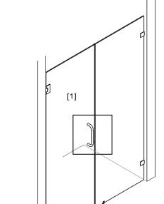
7. Install the Handle Set[6] onto the Door Panel[1] with Allen Key.(Fig 1&2&3)
