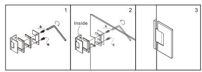
2. Remove the screws from the Hinges[7].(Fig 1)
