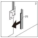
4. Cut the extra part of Side Gaskets[3], and make the top of Side Gaskets[3] aligns with the top of the the glass after assembled.(Fig 1)
